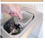
Place container into machine and swing the suction pipe down
