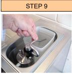
Place container into machine and swing suction pipe down
