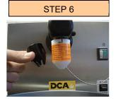
After cycle cream nozzle and place into container. Attach cleaning nozzle.
