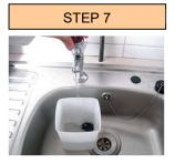
Wash cream nozzle under hot water. Fill container with hand hot water (around 50C)
