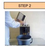
Remove and wash cream container. Place waste bucket under nozzle.
