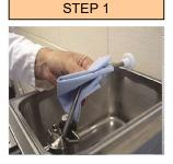
Remove lid, whilst lifting suction pipe wipe clean.
