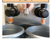
After cycle remove cream nozzles and place into container. Attach cleaning nozzles
