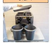
Remove lid, place waste buckets under nozzles
