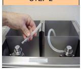
Remove connectors with tubes attached. Place into containers. Disassemble, wash parts and containers. Reassemble tubes.
