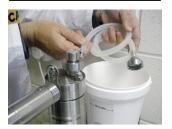
Remove connector with suction tube attached, place into cleaning bucket.
