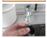
Wash cream nozzle under hot running water and place into cleaning bucket
