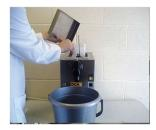
Remove and wash cream container. Place waste bucket under nozzle.
