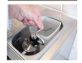
Place container into machine and swing the suction pipe down
