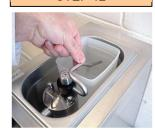
Place container into machine and swing suction pipe down
