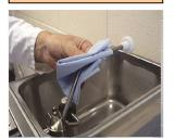
Remove lid, whilst lifting suction pipe wipe clean.
