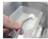
Place cleaning bucket into machine and swing suction pipe down
