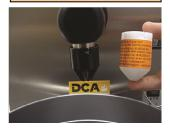
After cycle remove cleaning nozzle. Reattach cream nozzle. Remove cleaning nozzle
