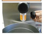
After cycle remove cream nozzle and place into cleaning bucket.
