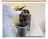
Return cream container to machine. Replace lid. Switch on refrigeration (green button)
