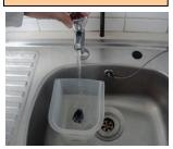
Wash cream nozzle under hot water. Fill cleaning bucket to level line with hand hot water (around 50°C).
