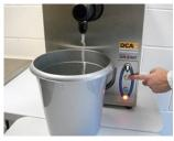
Switch off refrigeration (green button). Press cleaning button once. Auto pre-rinsing begins (2 mins).
