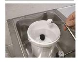
Place cleaning bucket into machine and swing suction pipe down
