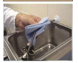
Remove lid, while lifting suction pipe & wipe clean.
