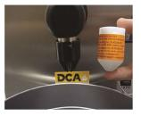
After cycle remove cleaning nozzle. Reattach cream nozzle. Remove cleaning nozzle
